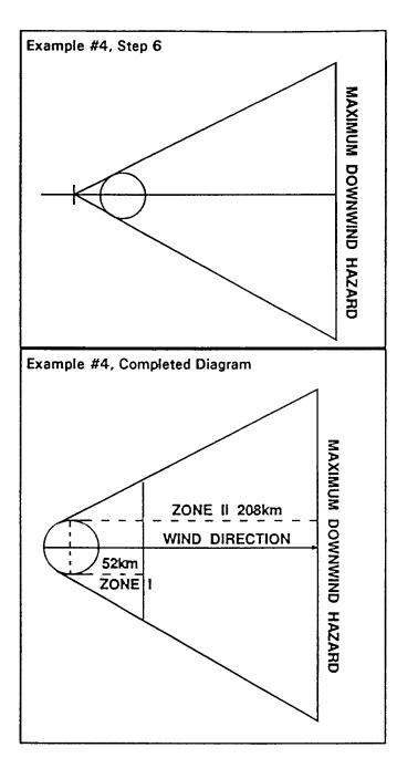
5. Draw a perpendicular line intersecting the MDWHD point on the representative wind direction line drawn from the attack area endpoint furthest downwind (This is the line of Maximum Downwind Hazard example #6, step 4).
